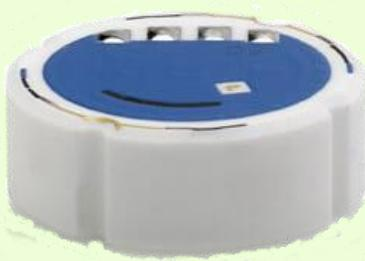
The gauge uses a solid ceramic pressure sensor made of aluminum oxide ceramics from Metallux (Switzerland). On one of the inner sides of the sensor is a thick-film membrane. The housing contains contacts for connecting the wire leads. High accuracy of the sensor achieved through laser matching of the resistive bridge and temperature compensation. As a result, the error of the
