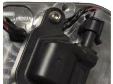
Install and tighten all button heads firmly at this time.
