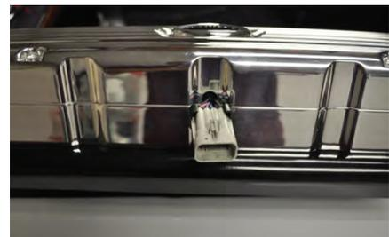
Apply Anti-Seize to the threads of the 1/4-20 X 1-1/4 ARP 12pt. cap screws. Install top billet coil cover carefully not to pinch coil harness and tighten.
